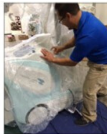
Step 3. Remove tape from 36" x 44" drape sheet and attach over column to main body and bumper assembly.
