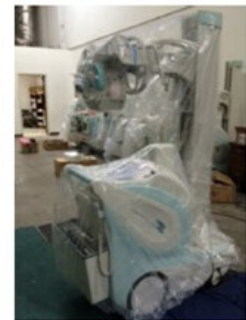
Step 3. Remove tape from 36" x 44" drape sheet and attach over column to main body and bumper assembly.
