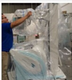
Step 2. Remove 42" x 120" bag and place over fully extended XR tube and column
