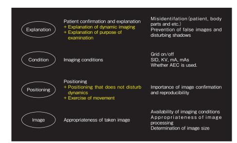
Fig. 1 Procedure Flow of DDR
